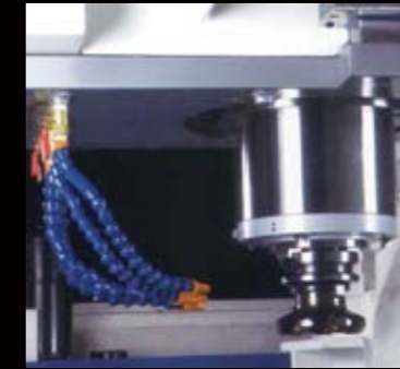
Spindle head and coolant nozzle ring
