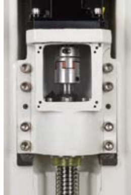
Strong direct drive coupling with pre-loaded ball screw
