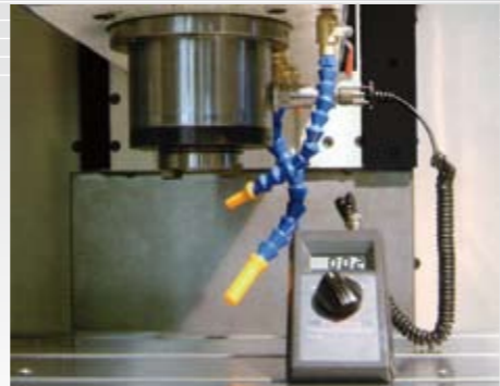
Vibration test of spindle
