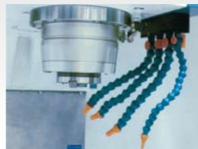
CTS Coolant thru spindle (OPT.) ATS Air thru spindle (OPT.) Coolant nozzle in spindle head (STD.) Spindle air purge (STD.)
