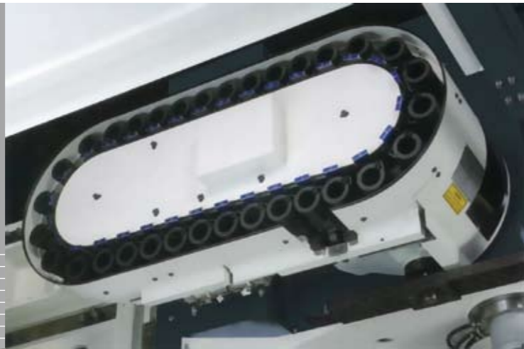
Swing arc ATC with 32 tools position (MV1750S-STD)
