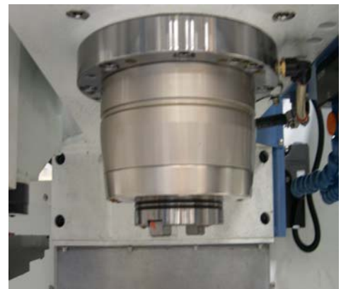
Picture 2: no tool in the spindle
